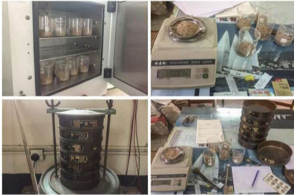
Figure 2-14: Photograph showing the grain size analysis in laboratory
