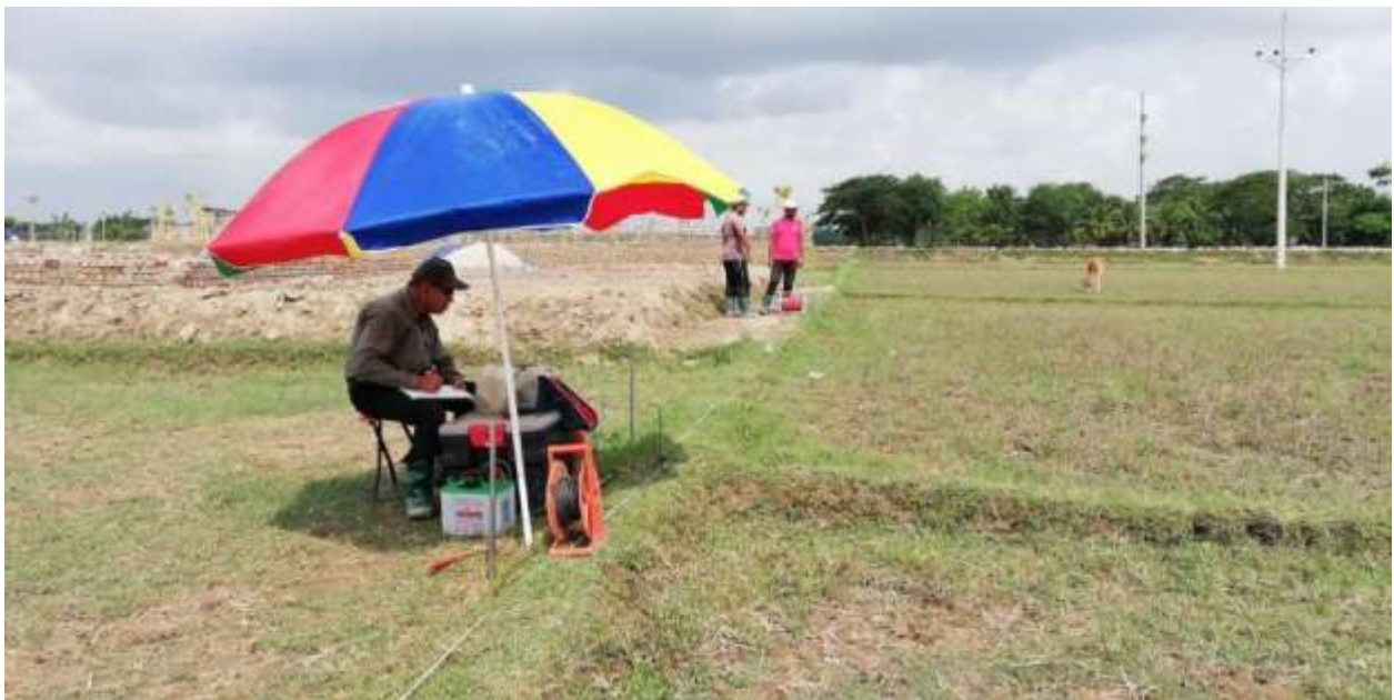
Figure 2-12: Resistivity Survey [Vertical Electrical Sounding (VES)]
